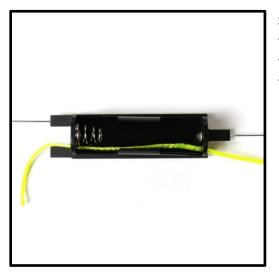
**Step 1** - feed your flight line through the two round holes in the ends of the battery case. Make sure you feed it through the bottom hole first and then the upper hole (the hole by the GPS antenna). It is easiest to perform this step with the battery removed.
