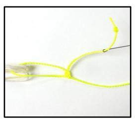
Step 3 – feed the remainder of the flight line through the loop in the upper antenna wire and tie a stopper knot. Our favorite stopper knot is the figure-eight knot. Make sure the stopper knot can't pull through the loop in the end of the antenna wire. If it does, use thicker flight line. This keeps the StratoTrack from Sliding down the flight line towards the payload. Verify that the GPS antenna is pointing up and not down when the balloon lifts the flight line vertical.
